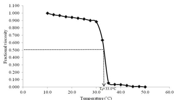
Figure 4. The thermal denaturation curves of pepsin-solubilized collagen (PSC). The denaturation temperature ( $T_d$ ) of PSC was 33°C.
